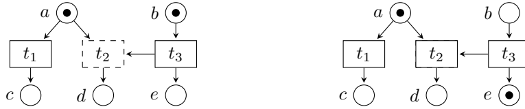
(a) The initial net D_0 . The transition t_2 is not initially available to be fired.
